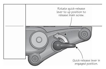
Figure 11: Releasing the half nut.
