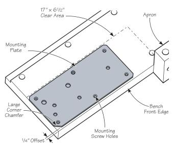
Figure 4: Aligning mounting plate and transferring screw hole locations (right-hand mounting shown).
