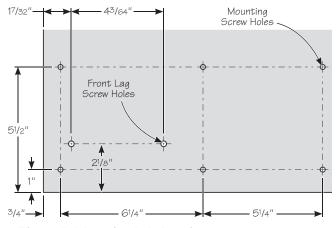
Figure 5: Mounting hole locations.
