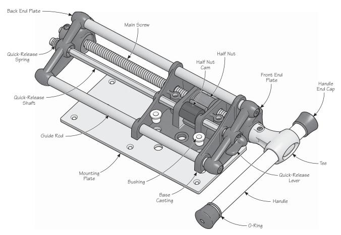
Figure 1: The Veritas<sup>®</sup> Quick-Release Tail Vise mechanism, shown upside down.
