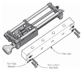
Figure 3: Attach jaw to mechanism.
