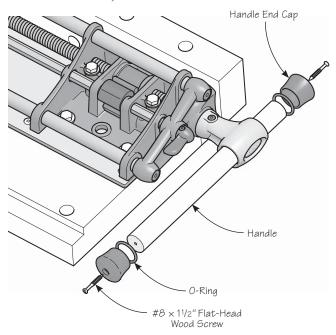
Figure 9: Installing the handle.
